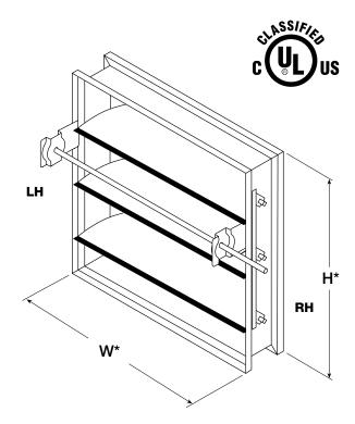
\*W&H dimensions furnished approximately 1/4 in. (6mm) undersize. (Add sleeve thickness for overall sleeved damper dimension)
